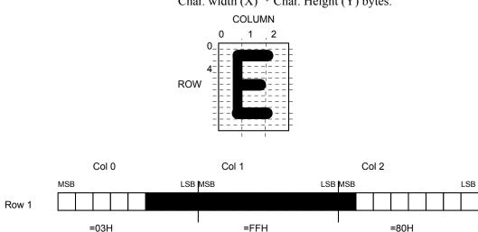
The bitmap data consists of bitmap patterns for each character in a character set for which the parameter Char width in the Char matrix table is set to a value between 1 and 24. A character that has its Char width set to zero, is not included in the bitmap data.
